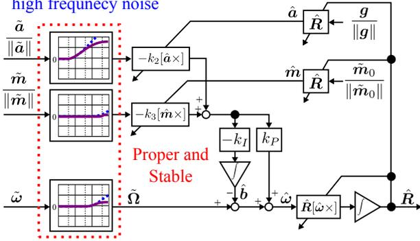
(b) Explicit complementary filter with filtering the measurement by the inverse transfer function which is made proper and stable by the relaxation of the complementary condition
