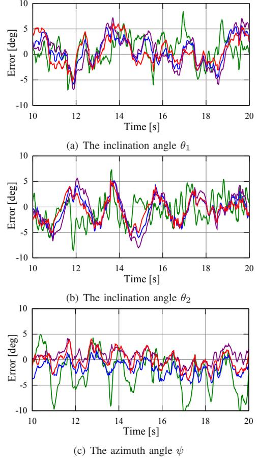
Fig. 5. The enlarged view of an example of the estimation errors from 10.0[s] to 20.0[s]. (Red line is the proposed method, green line is the authors' previous method, blue line is ECF, and purple line is Pro. wo. EVF.)
