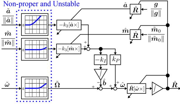
(a) Explicit complementary filter with simply filtering the measurement by the inverse transfer function
