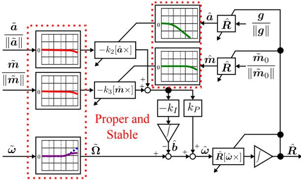
(c) The proposed method which only uses the proper and stable transfer function by the relaxed complementary condition and the sensor dynamics filtering of the estimate fed back to the error computation
