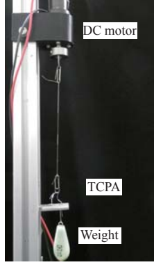
Fig. 2. The machine to fabricate TCPA. TCPA is fabricated by twisting DC motor attached on the upper end of the nylon thread.
