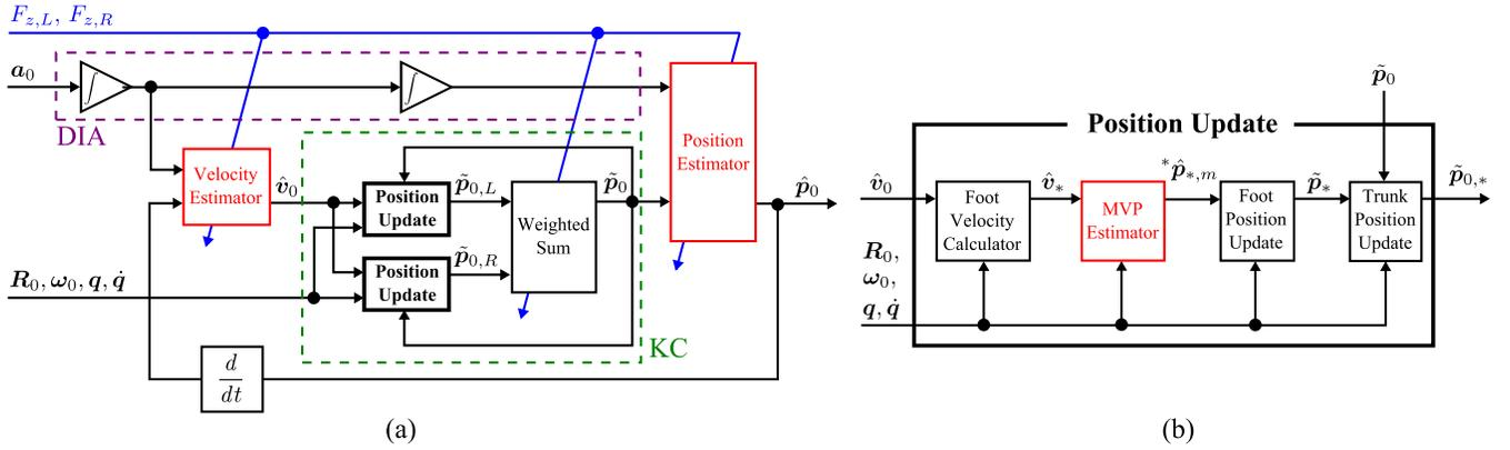
Fig. 1. The proposed dead reckoning (a)the overview of proposed dead reckoning(the red box is the estimator, the green and purple box denote KC and DIA, respectively, and the blue arrow is the reaction force). (b)the detail of "Position Update"(the red box denotes MVP estimator)
