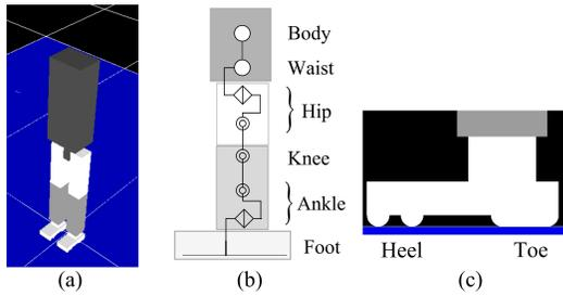
Fig. 3. Robot model for simulations (a)exterior (b)kinematics (c)side view of the foot
