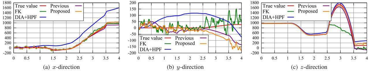
Fig. 8. A result of position estimation for jumping. (The vertical axis is position[mm] and the horizontal one is time[s].)
