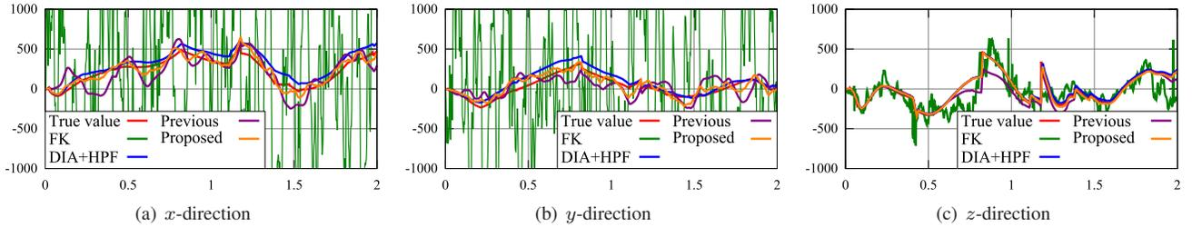
Fig. 6. A result of position estimation for walking on the plane. (The vertical axis is velocity[mm/s] and the horizontal one is time[s].)
