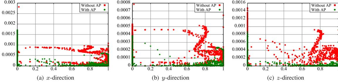
Fig. 4. The relationship between the absolute value of position errors of the kinematics computation from the left foot (vertical : [m]) and  $\hat{f}_{Lz}$  (horizontal).
