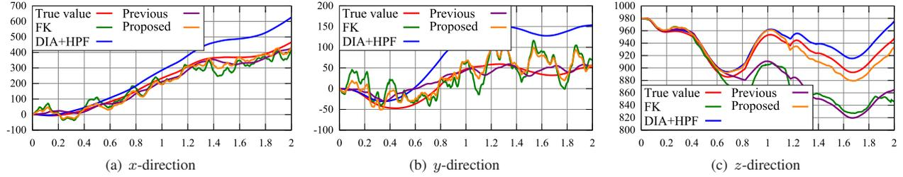
Fig. 5. A result of position estimation for walking on the plane. (The vertical axis is position[mm] and the horizontal one is time[s].)
