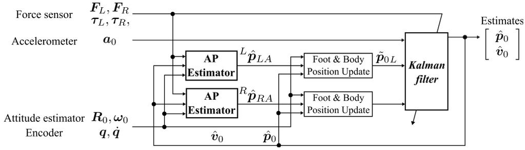
Fig. 1. The proposed Kalman filter
